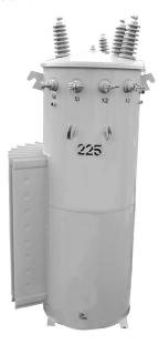
Triplex overhead distribution transformers are often used to serve large motor loads where the motors are frequently started. Oil field pumping loads and some irrigation pumping loads should use only triplex designs. Also, the Triplex transformer has international applications where Dy 5 and Dy 11 phase displacement are required.
